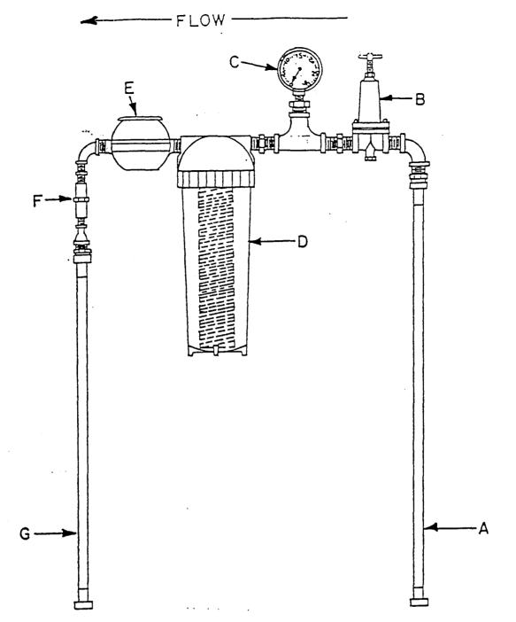
Figure 1. Water Sampling Device
